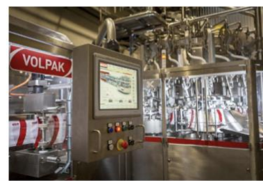
Volpak SC+ machine is a continuous movement horizontal form fill seal unit. (photo: Volpak)
