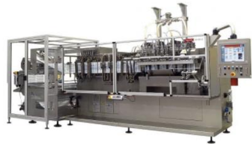
The SP 170: a Volpak machine for pouch forming and filling. (photo: Volpak)
