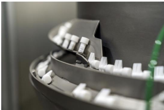
Detail of the Enflex F-11 machine especially suited for the healthcare sector for the packaging of a wide range of products. (photo: Volpak)
