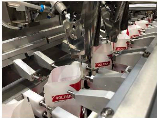
Volpak will showcase the new SI 280, a horizontal form fill seal machine.
